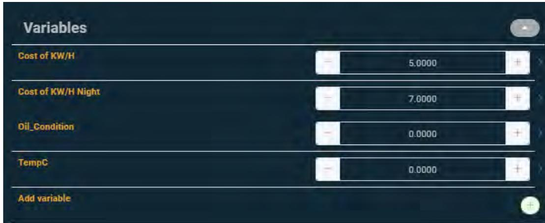
Other examples above are **Oil\_Condition** and **TempC**. The value should be left at 0 if the data from a Phantom sensor is used as the variable. In this case, a T25 Temperature Phantom is configured in the *item* Child 1. The input unit is set to temperature in C. The latest value reported from the sensor is stored in this variable, e.g. 32 for 32 degrees C.
