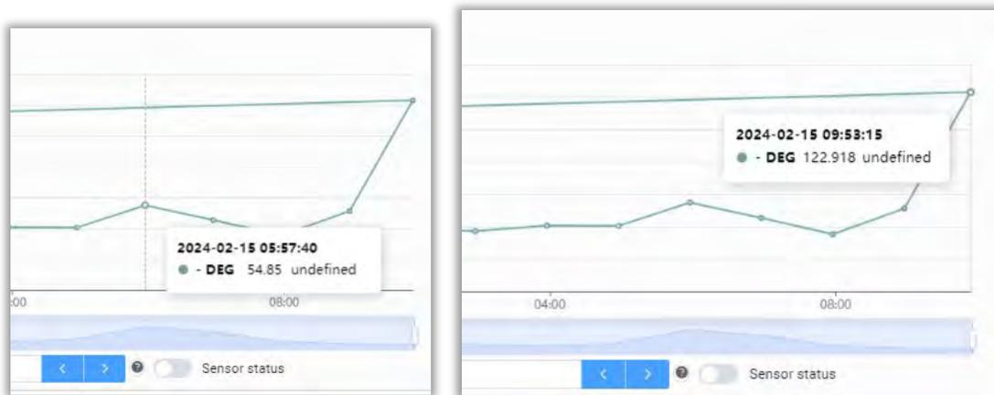
After applying the **Convert to F** function to this item, the temperature is now displayed in Fahrenheit for subsequent measurements.
