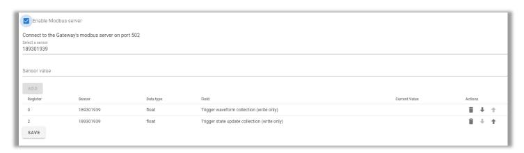
In this example, when the Modbus server writes a "1" in register 0, it will trigger a waveform collection. If a "1" is written into register 2, an RMS update will be sent.
